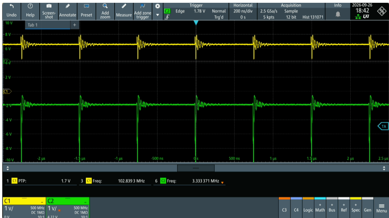
Figure 7: Code-timed (I can hear the CS-bro’s screaming) DDS doing on-the-fly floating-point sine calculations but without SPI transactions, roughly simulating parallel I/O maximum sample rate of about 3.333 MSPS. Some bro-grammers will also call for DMA, which does not work for DDS (except for pushing pre-computed blocks of data), but works like a champ for fixed-table synthesis (coming soon to a tutorial near you!).
