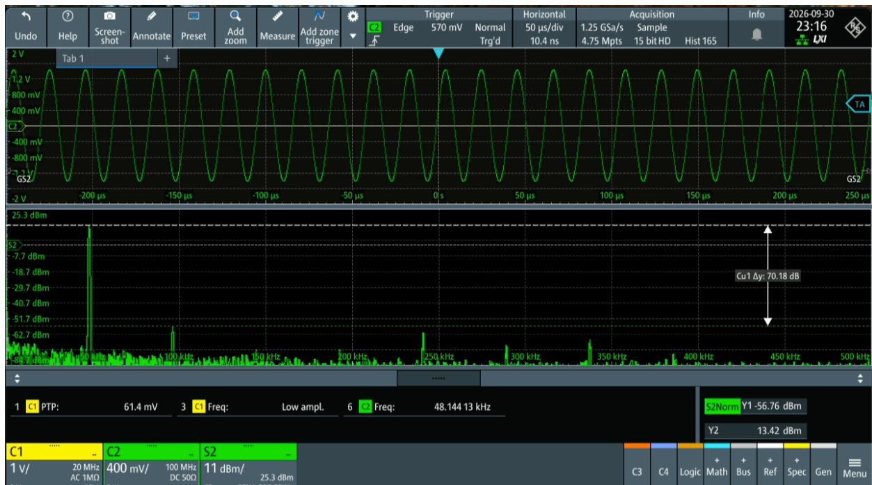
Figure 13: 10kHz, 3VPP, 76.2 dB SFDR, not bad! But never believe an SFDR close to that of the ADC in the scope... 😊
