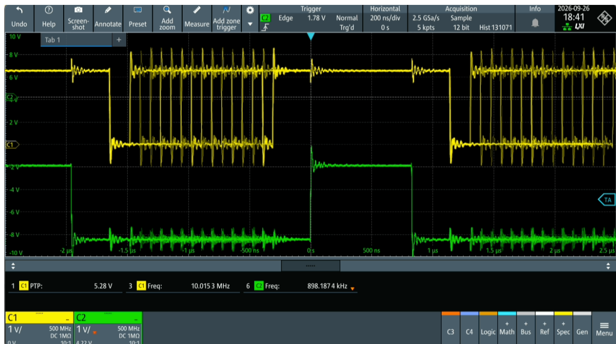
Figure 6: Testing “On-the-Fly” DDS with hardware SPI on Teensy 4.1 – this is not limited appreciably by the way sine() is computed, by the way. With the constant-time arm_sin_f32() function it edges up to 1MSPS with 30MHz SPI clock.
